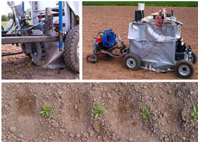
Lukas - Robotic mechanical weeder for ecological cultivations
